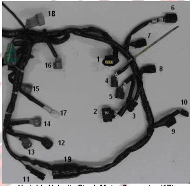
Variable Velocity Stack Motor Connector (17)
